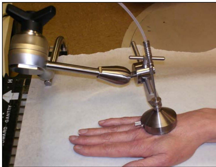
Photograph of the horizontal (H30) and perpendicular (V30) Leipzig applicators with a 30 mm cone diameter.
